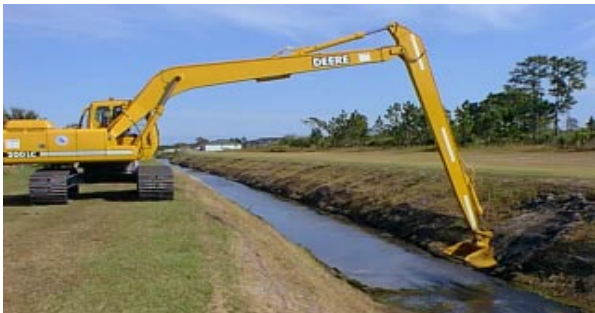
The City's new track hoe, purchased for $165,000 in October, is put through the paces by operator Donnie Farnham. This new equipment can clean 1,000 feet of large canals per day compared to the 100 feet per day achieved by the drag line it replaces. The machine is a mechanical excavator that moves on metal tracks instead of wheels.
